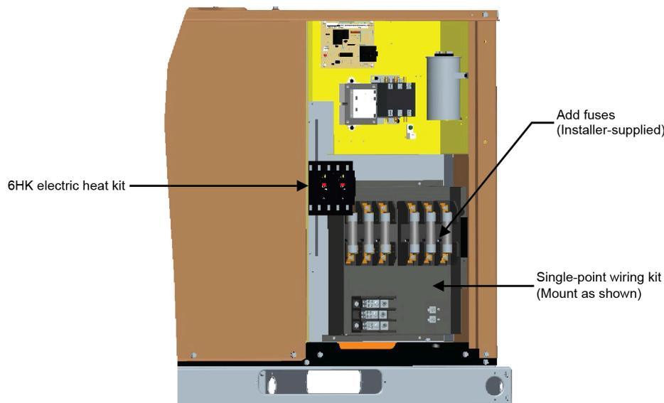
To install a single-point wiring kit, do the following:
