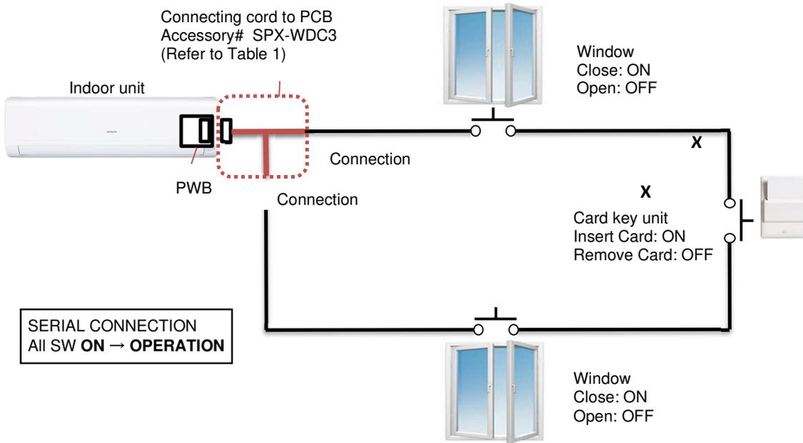
ii. Pin No. 3 of DIP SWITCH is set to ON position (LO Input Active) for Dry Contact Type b
