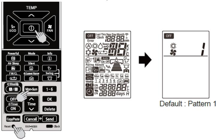
2. Press [ROOM TEMPERATURE setting] [^(UP)]/[V(DOWN)] buttons. (The intermittent pattern changed with indoor unit beep sound.)
