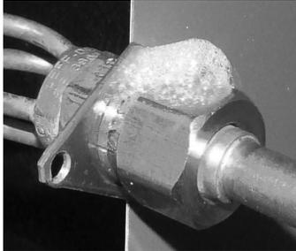
2. Check all brazed and screw-on line connections by applying a soap solution to the joint. A leak will produce bubbles in the soap solution.
