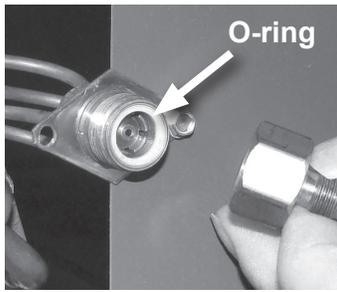
I-2. Replace the Teflon O-ring (located between the halves). Discard Schrader if present.
