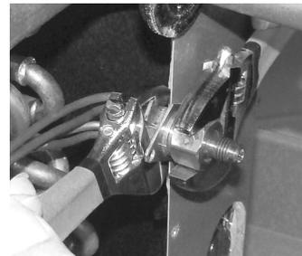
I-1. Disassemble flowrator body using two wrenches and unscrewing with a counterclockwise motion.
