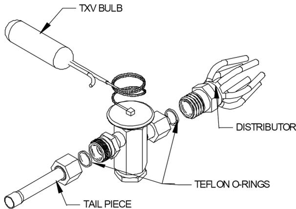
Fig 7B-1. Components of a typical TXV assembly
