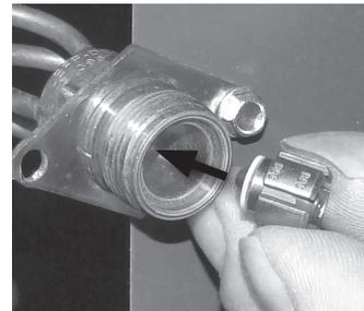
II-6. Replace the piston with one of the correct size. Do not force the new piston into the body. Make sure the piston moves freely in body.
