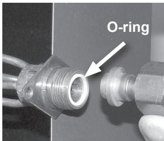
I-5. Taking care that the white Teflon seal is still in place inside the flowrator body, firmly seat the stub and screw the attachment nut to flowrator body.
