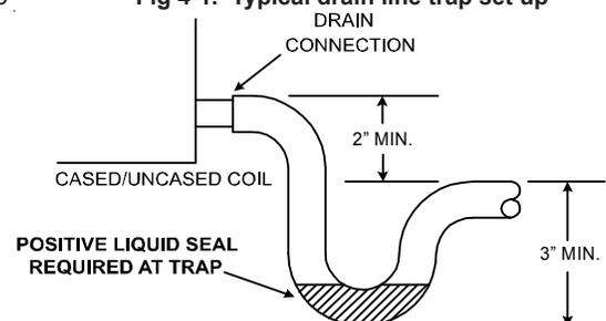
**CAUTION** Use Teflon tape to connect the drain lines to the threads in the drain pan. **DO NOT USE SOLVENT BASED PIPE DOPE. THIS WILL REDUCE THE LIFE OF THE PAN.**
