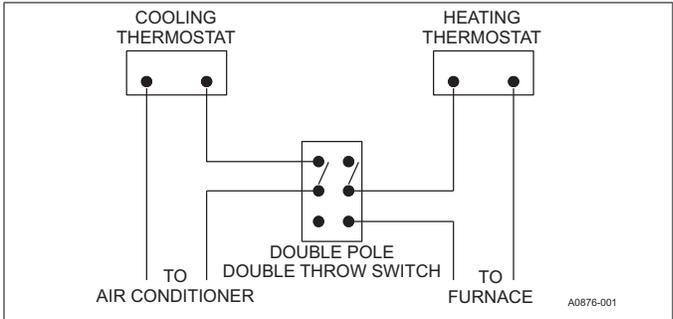
FIGURE 12: Thermostat Wiring
