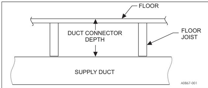
**FIGURE 4:** Duct Connector Depth (7990 Series)
