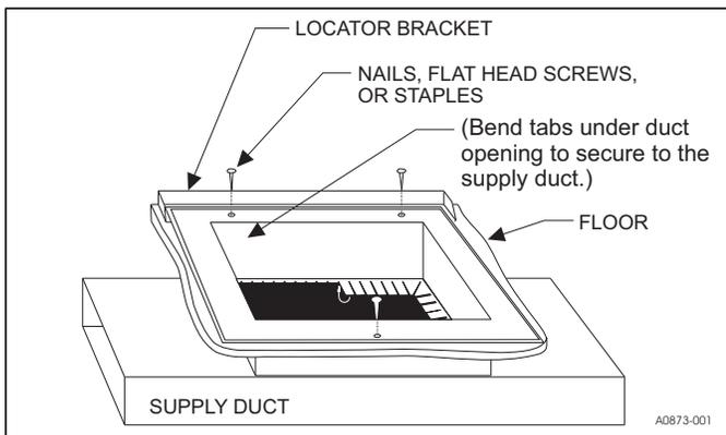
**FIGURE 8:** Duct Connector Tab Attachment (7990 Series)
