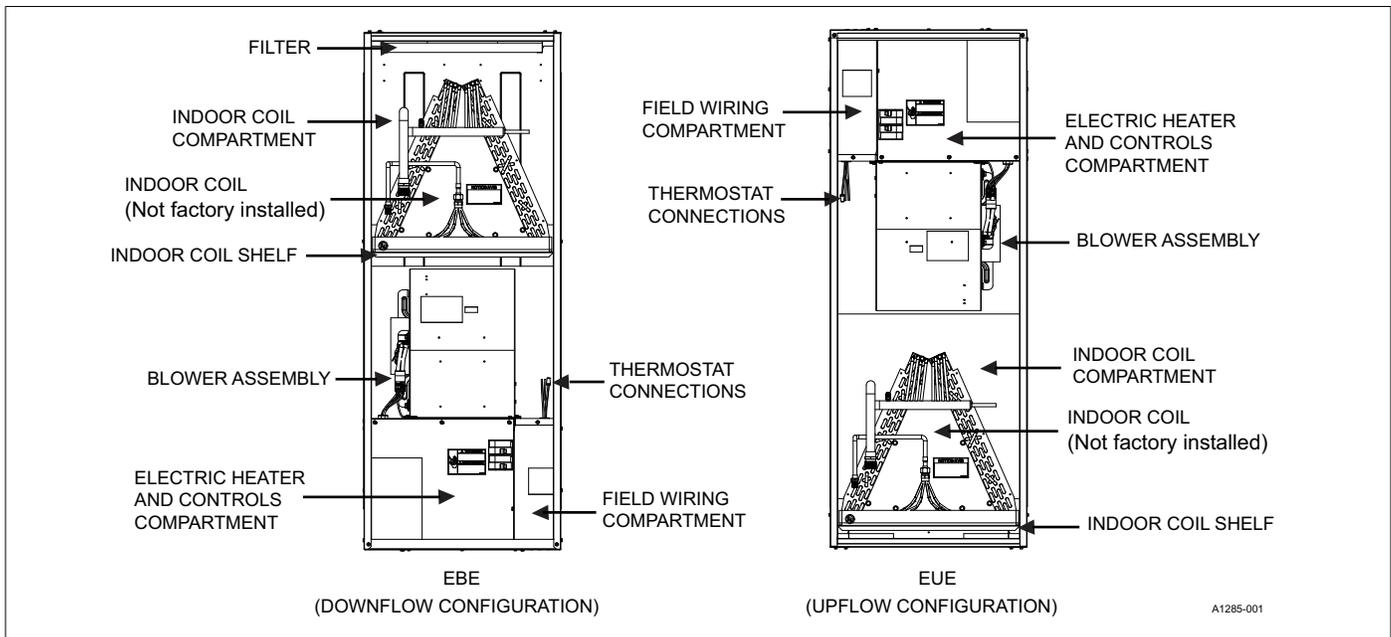
FIGURE 13: EBE/EUE Furnace - Location of Components
