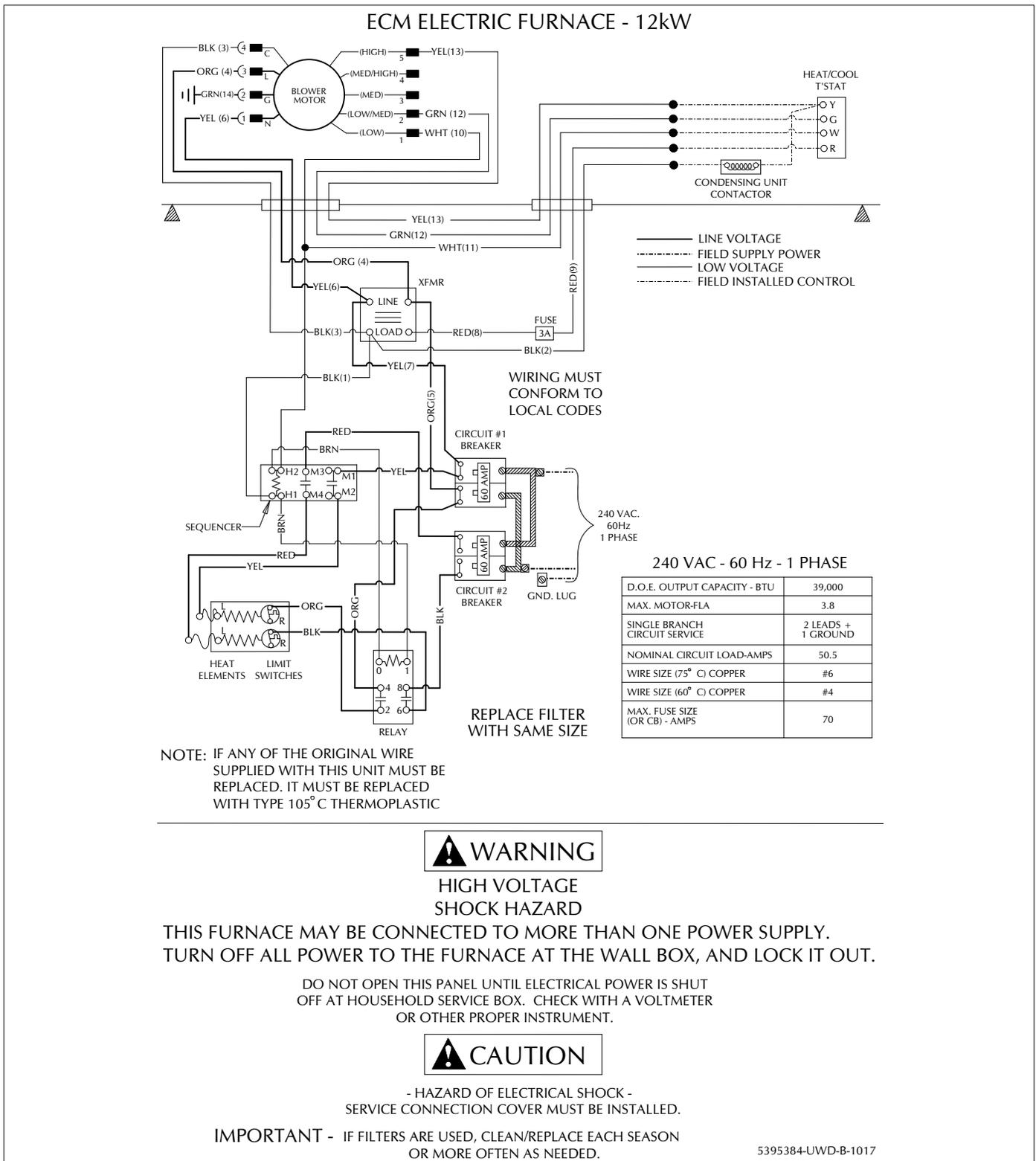
FIGURE 15: EBE12\*/EUE12\* Wiring Diagram
